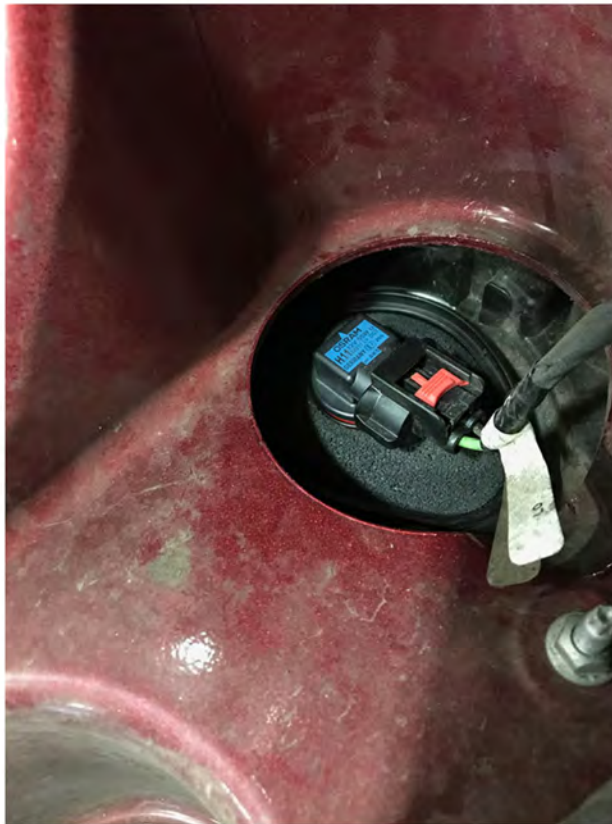
Fig 407, Correct Halogen Headlamp Installation With Foam Grommet
