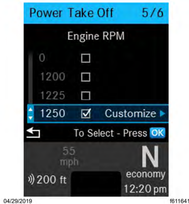
Fig 71, Quick Access Screen: Power Take Off (PTO)
