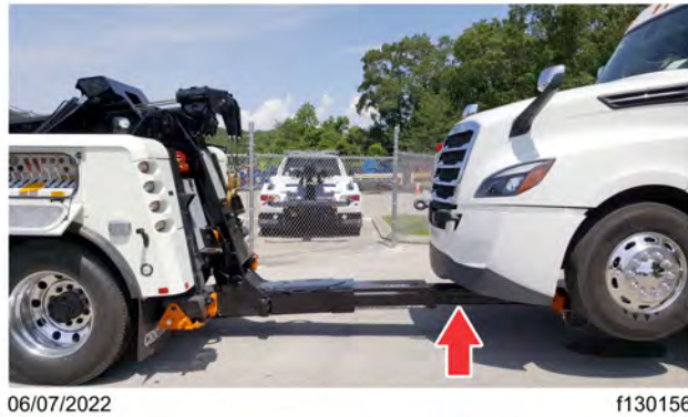
Fig 433, Retracting the Recovery Boom
