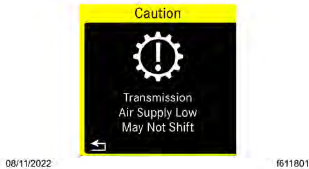
Fig 359, Low Transmission Air Pressure Pop-up
