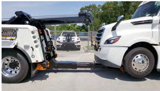
Fig 432, Stinger with Lift Adaptors Under the Axle (tow truck shown)
